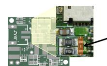
Cut area to set charge current R300 + R100: ~1866mA R300: ~1400mA R100: ~466mA
