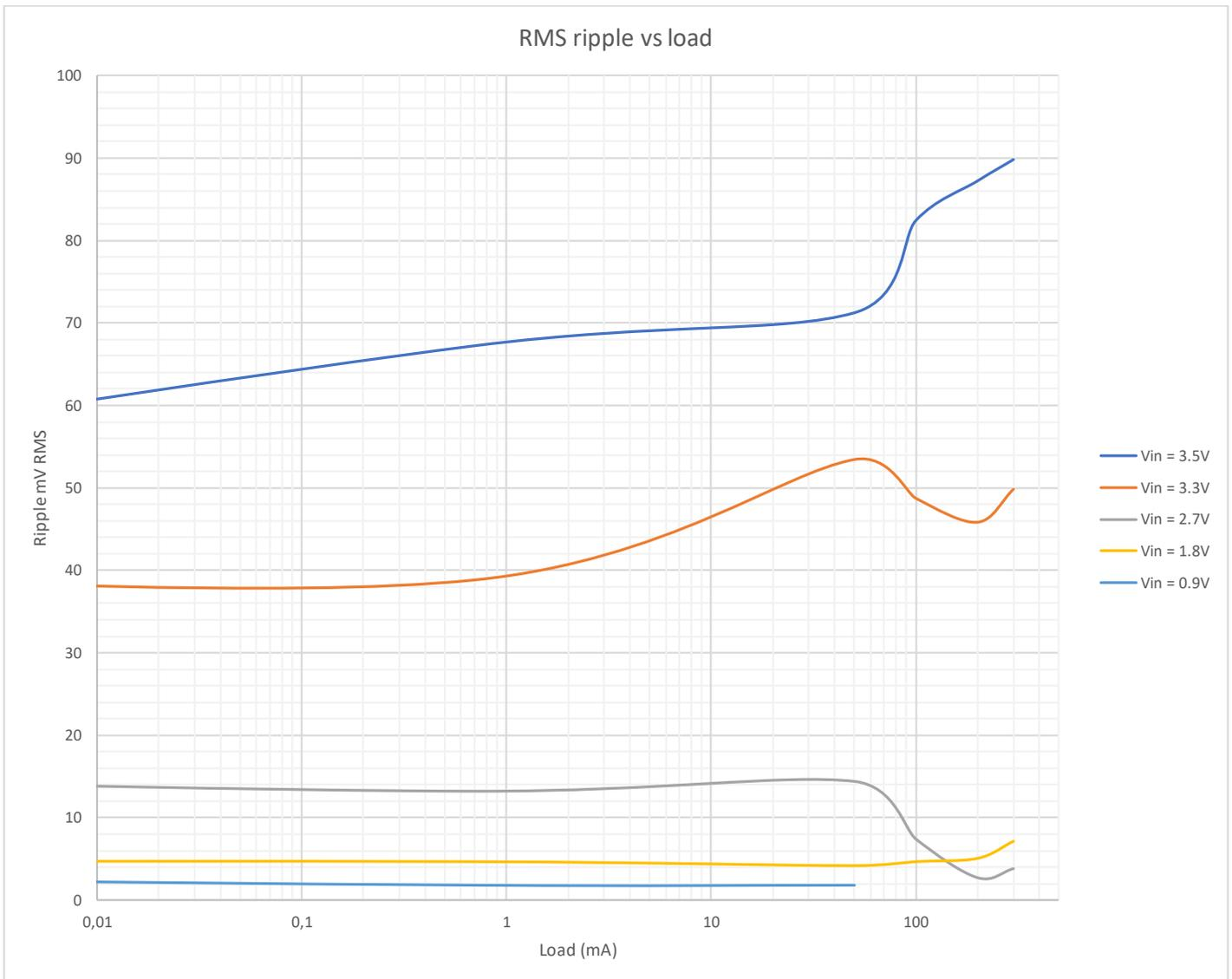
Note: measured at 20MHz bandwidth using a 1x probe.
