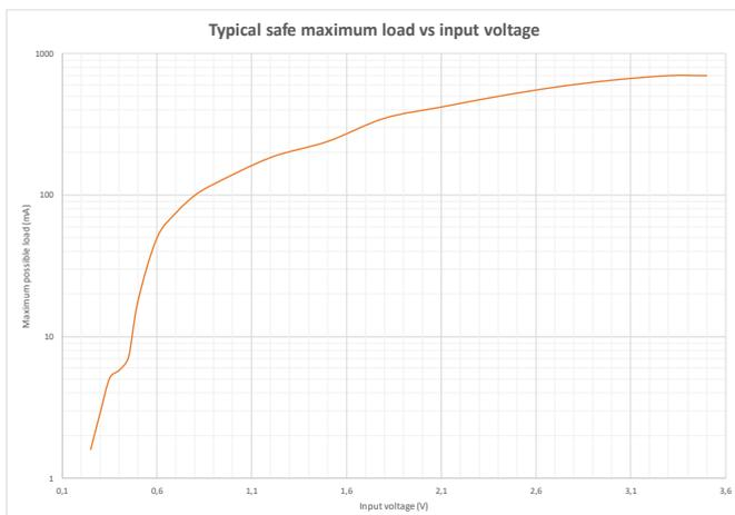
Exceeding the operation range displayed in the chart may result in loss of regulation or overheating of the module.
